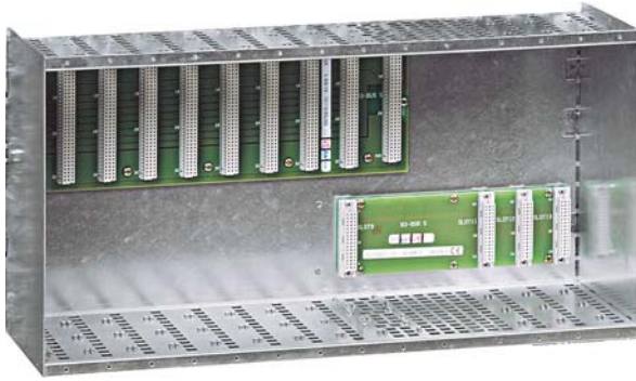
Empty module rack with BUS-circuit boards
